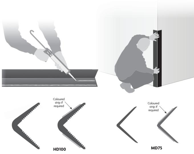
**HD type** Corner Angles measure externally 100 x 100mm. **MD type** Corner Angles measure externally 75 x 75mm.
