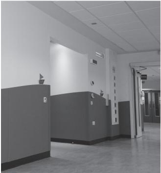
If the wall surface is unsuitable for fixing with double sided adhesive tape, we recommend using **Yeoman Shield 2000** Polymer adhesive. A run of double sided adhesive tape should be applied to the top edge of the panels to hold it in position while the mastic cures.
